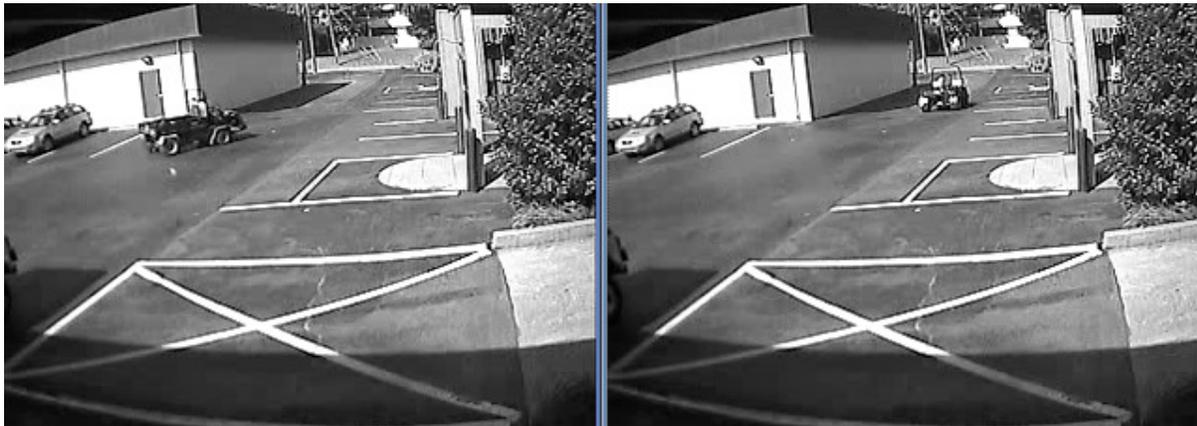
The next figure shows a PixMin™ client display of the final frame, when operating in highlight mode. PixMin™ marks objects at their current location and tracks their motion back to recent locations. Besides highlighting events in this way, the PixMin™ client triggers audible and visual alerts.
