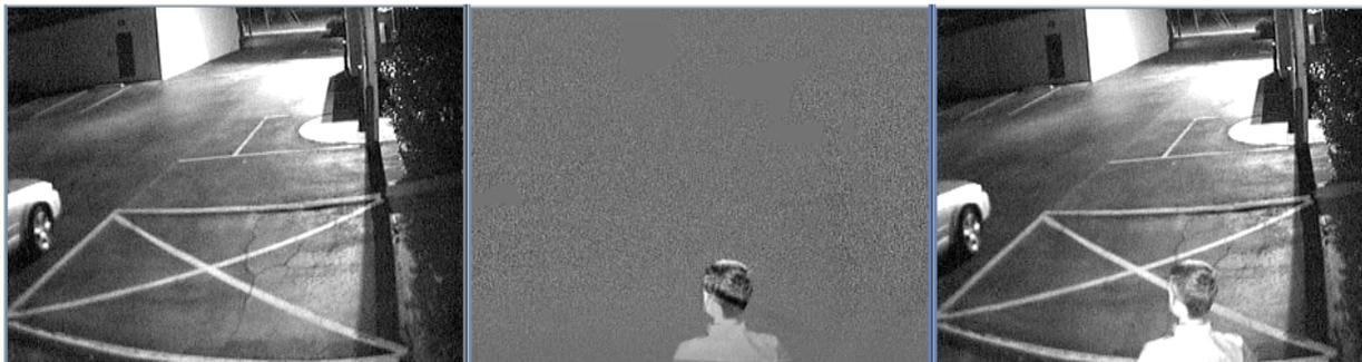
The above figure shows how PixMin™ data reduction works. The frame on the above left shows a reference frame that PixMin™ transmitted and saved in full resolution. The frame in the middle shows interesting pixels that the PixMin™ server identified. The frame on the right shows the resulting, fully recovered PixMin™ display.
